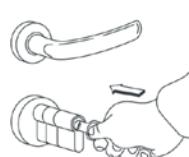
7) Securemme cylinders are equipped with projecting cam lever to offer a better hold in the event of breakage. It is possible to insert and remove the cylinder from the lock without destructive operations, only having available the keys or by turning the knob.
